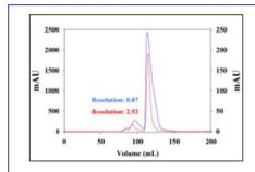
Overlaid chromatograms from the pSEC step representing the extremes of observed resolution. For the sample with good resolution (red), the loading volume was 2mL, at a concentration of 2mg/mL, and ran at a flow rate of 5mL/min. The sample with poor resolution (blue) used a loading volume of 8mL at a concentration of 12mg/mL, and was ran at a flow rate of 10mL/min. The resolution between monomer and aggregates as calculated by UNICORN software is shown.
